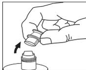
Unscrew plastic cap and remove plug from threaded end of cartridge. Save cap and plug to reseal if entire cartridge is not used.
