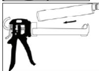
Place cartridge into a 10 oz. caulk gun. Rust-Oleum #257396 Heavy-Duty Caulk Gun is recommended (26:1 ratio minimum).
