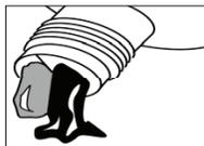
Dispense a small amount of adhesive into a disposable container until both materials flow from cartridge.
