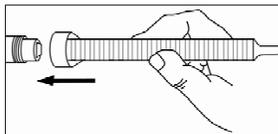
Attach mixing nozzle to cartridge and dispense a small amount of material into same disposable container until a consistent color with no streaks is obtained.
