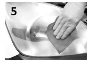
Tear open the Wipe-It™ packet, pull out the applicator cloth and carefully wipe the lens ONE TIME, being careful not to get any Wipe New® onto the surrounding paint. If treating multiple lenses, do so before the Wipe-It™ dries out.
